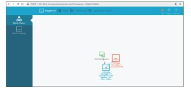
(3) If the third X5000R joins the EasyMesh network, for the connected slave device, follow the third step again to set up the slave device environment. Then simultaneously press and hold the WPS/RST button of the master and slave device for 1-3 seconds to continue sending the networking request. During the trigger period, a new network will be added after the response is received.(Required waiting for 2 minutes.)
