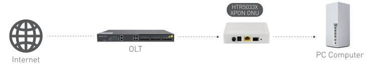
Figure: HTR5033X Application Diagram
