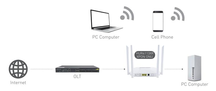
Figure: HUR4113XR Application Diagram
